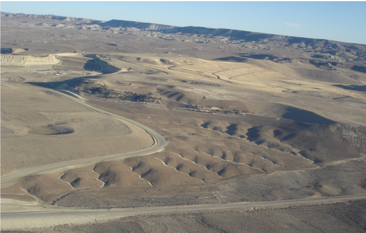
AERIAL VIEW OF THE COMPLETED STEEP SLOPE NATURAL REGRADE IN FOREGROUND – TRADITIONAL 4:1 RECLAMATION SLOPES WITH CONTOUR DITCHING IN DISTANCE
