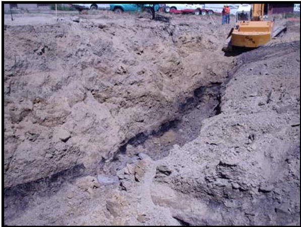
Canyon View Evidence of Subsidence 3' Offset of Coal Seam:
