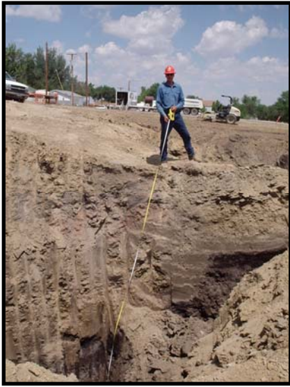
Canyon View Evidence of Subsidence 3' Offset of Coal Seam:
