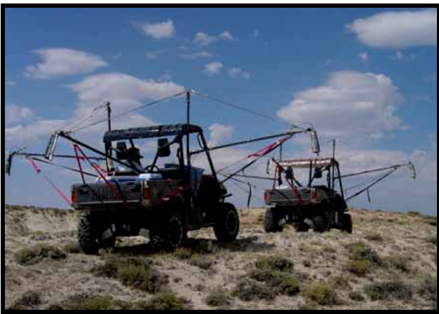
Photo 15: Three detector OHV system utilized for baseline radiometric surveys
